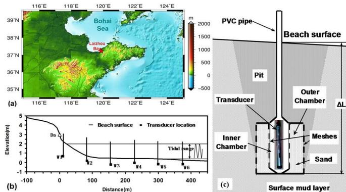
Figure 1. (a) Location of the studied tidal flat in Laizhou Bay of Bohai Sea, China. (b) Locations of W1-W6 along transect. (c) Schematic of transducer installation for measuring groundwater head.
