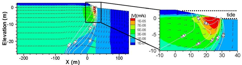
Figure 3. Darcy velocity (banded colored contours) in the transect averaged over a spring-neap tide cycle (about 35h). The arrows with uniform length are used to indicate the velocity direction only. White curves are contours of the pore water salinity.
