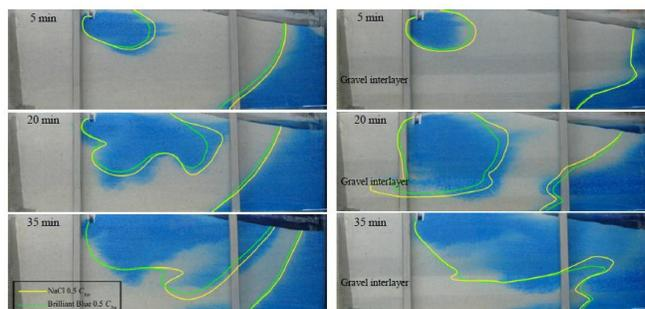
Figure 2. Contaminant transport results for simulation (lines) and experiment at low, medium and high tidal levels for (a) homogeneous sand and (b) sand with a gravel interlayer.
