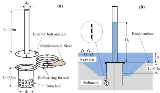
Figure 1. Schematic of (a) the apparatus, and (b) the in-situ installation of the apparatus for measuring hydraulic conductivity.
