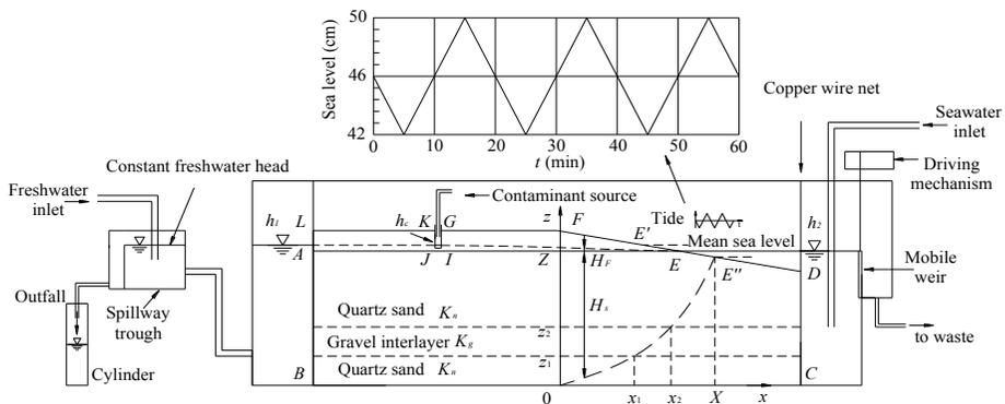
Figure 1. Sketch of the experiment setup. Tank is 160-cm long, 60-cm high and 10-cm deep.
