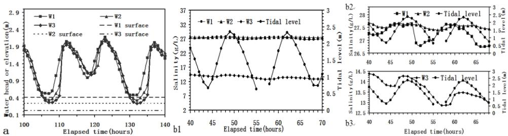
Figure 2. The initial time  $t=0$  h represents 17 September 2012, 11:00A.M. The sensor measured tidal level was placed above the beach surface at W1 and only the data during submergence was used. (a) Observed water head, tidal level and surface elevation at W1-W3 from  $t=100$  h to  $t=140$  h. (b) Salinity variations with time at W1-W3 from  $t=40$  h to  $t=70$  h.
