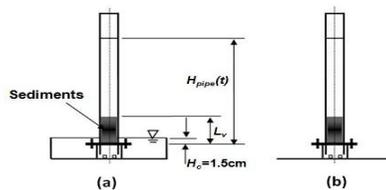
Figure 1. Schematic for two falling-head methods used. (a) Normal falling-head method; (b) Free drainage falling-head method.
