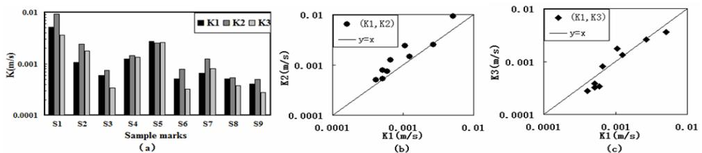
Figure 2. Comparison of  $K$  values of 9 samples.  $K_1$ : falling-head method,  $K_2$ : free drainage falling-head method; and  $K_3$ : Kozeny-Carman formula.
