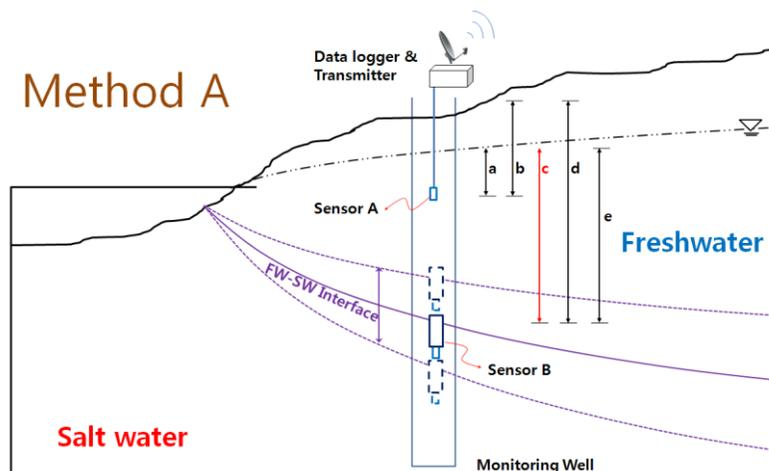
Fig. 1. Schematic description to get a time series data of the freshwater-saltwater interface location and thickness of the freshwater by using a floating device (B) and a fixed sensor (A).
