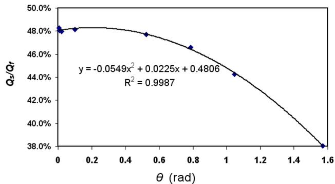
Figure2. Effects of  $\theta$  on the ratio when  $K=10^{-2}$ m/s,  $\alpha_L=10$ m,  $h_f=48$ m.
