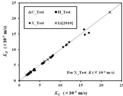
Figure 2. A plot of the  $K$ -values estimated by two methods ( $K_L$  is values of least-squares method, and  $K_D$ , values of finite-difference method). C\_Test, H\_Test, and X\_Test denote the tests at Caofeidian, Haimiao, and Xin Zhuang, respectively.
