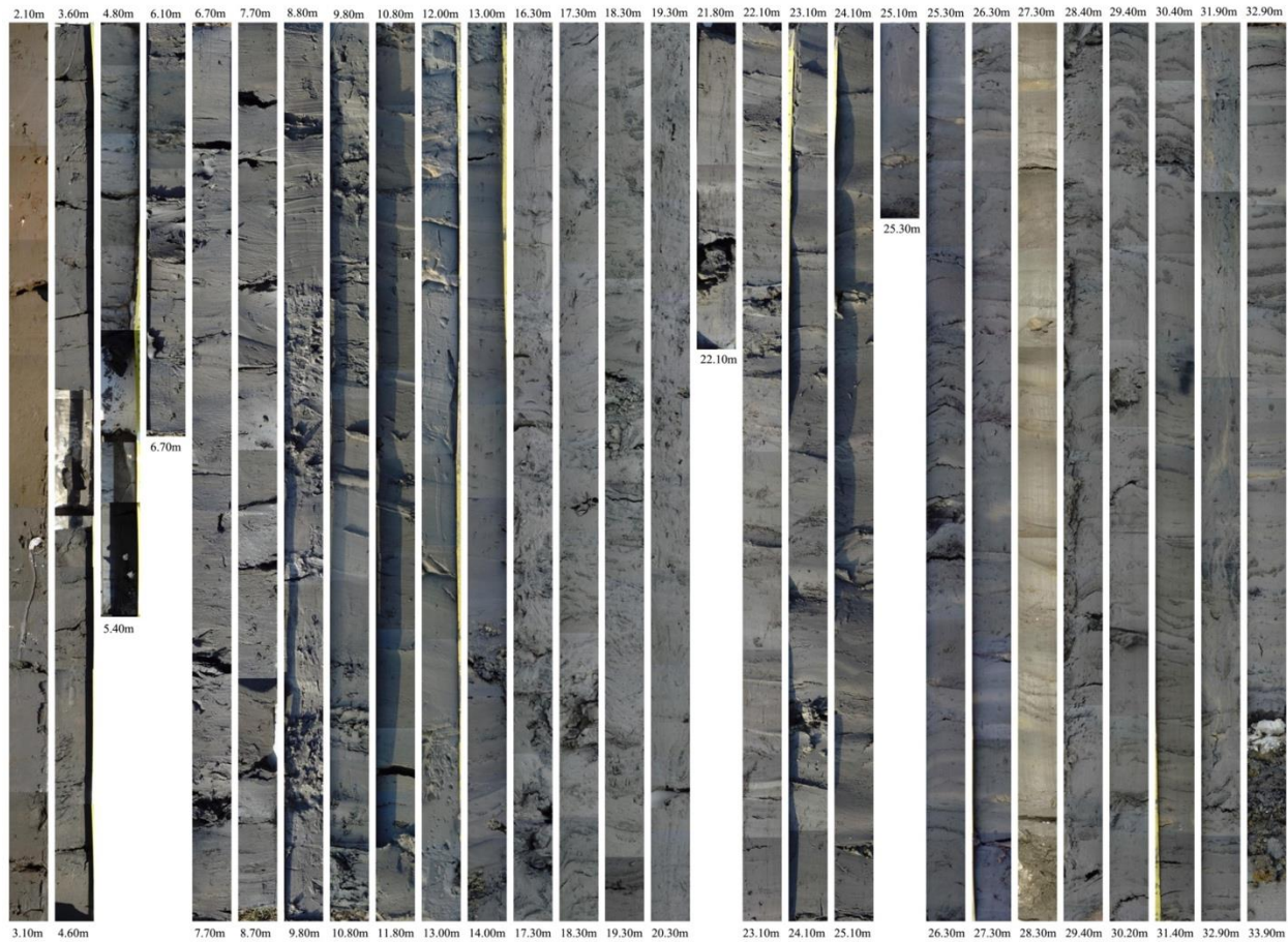
Fig 11 Image of cores from borehole in Mingzhong. It is hard to identify the materials change using naked eyes. Note the yellowish color from 27.30 m to 28.30 m was caused by the flashing of the camera when the photo was taken in the evening.
