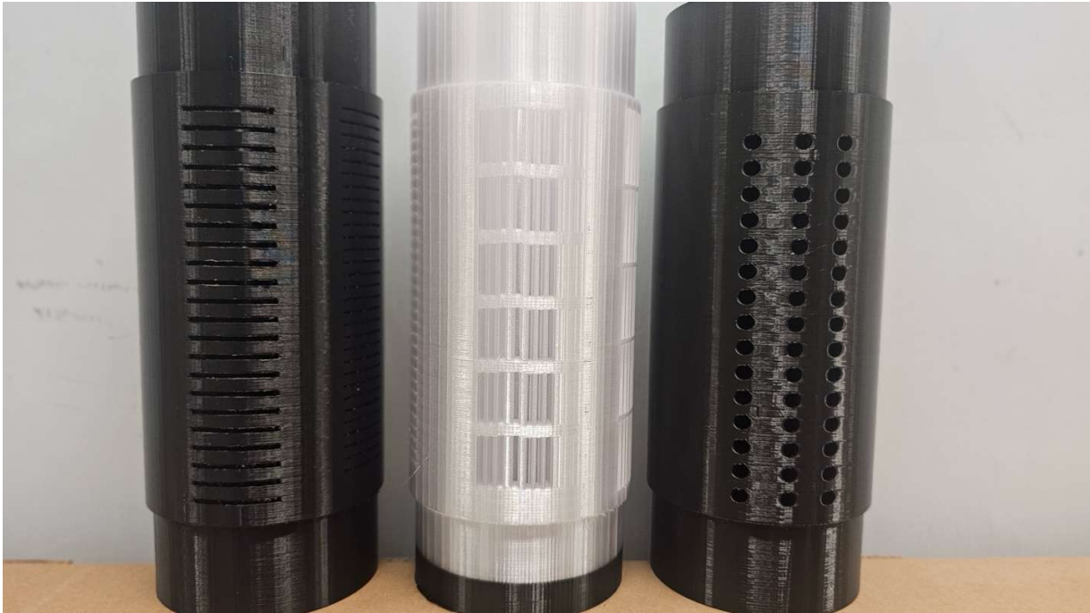
Fig. 3. Various designs of well screens tailored to meet the requirements of different geological formations. The screen section here is ~15 cm long and can be extended as needed.
